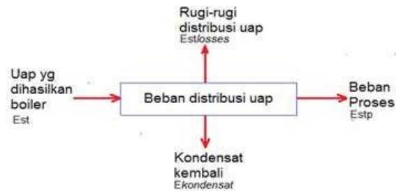
Figure 7. Energy balance in distribution load
