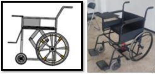
Figure 6. Wheelchair using hydraulic/triangle jack (left) and wheelchair-using hydraulic/bottle jack (right)
