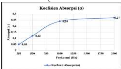
Figure 8. 25% Composite Absorption Coefficient Diagram.
