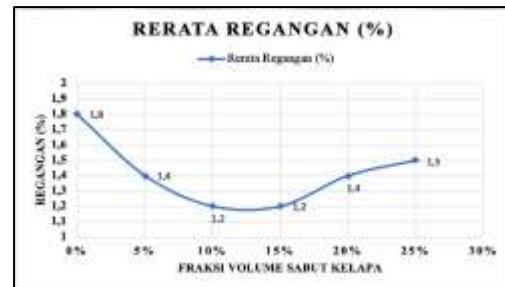
Figure 2. Strain Test Diagram
